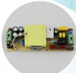
LED driver inside view
